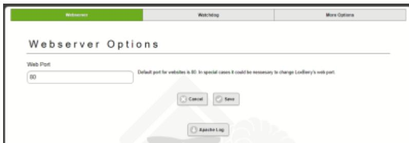
You can change the **Web port** of Apache from 80 to another free port, for example if the Homebridge plugin requires port 80. With the **Apache Log** button a live view of the Apache log is opened.
