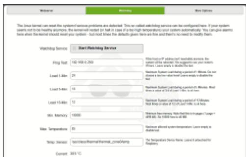
With the watchdog feature LoxBerry checks for important system health properties, and can automatically reboot, if thresholds exceeds.
