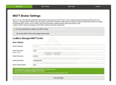
The default setting is to let LoxBerry configure and manage the locally installed MQTT Server. MQTT user, password and port are predefined.
