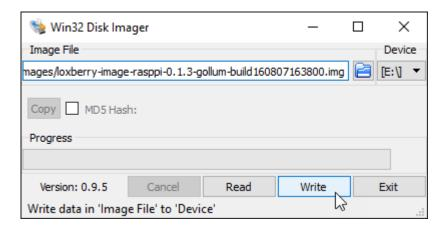
After the Success message, unmount the device and put the SD into your Raspberry Pi.
