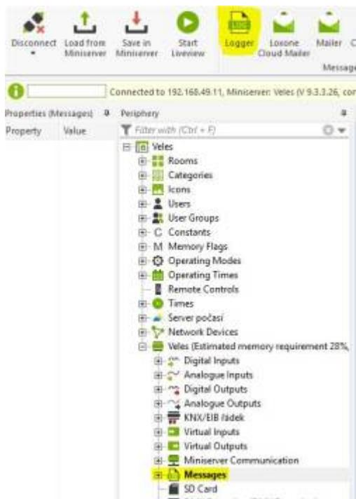
Logger is inserted. Fill name. In the "Address of Logger" fill something like "/dev/syslog/192.168.1.10". Use IP address of your LoxBerry!
